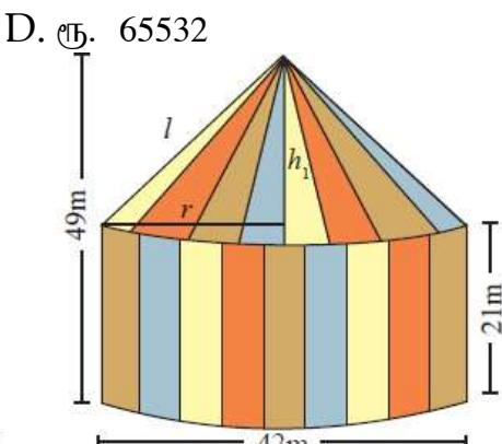
$$\begin{aligned}\text{Total area of the canvas needed} &= \text{CSA of the cylindrical part} + \text{CSA of the conical part} \\ &= 2\pi rh + \pi rl = \pi r(2h + l) \\ &= \frac{22}{7} \times 21(2 \times 21 + 35) = 5082\end{aligned}$$
