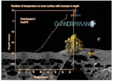
✓ ChaSTE measures the temperature profile of the lunar topsoil around the pole by means of 10 individual temperature sensors mounted on it.
