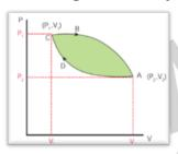
• The total work done is green shaded area in the figure. If the net work done is positive, then work done by the system is greater than the work done on the system. If the net work done is negative then the work done by the system is less than the work done on the system.
