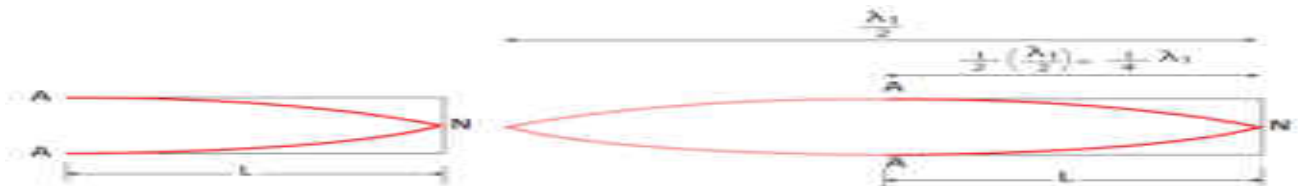
Figure 11.37 No motion of particles which leads to nodes at closed end and antinodes at open end (fundamental mode) (N-node, A-antinode)
