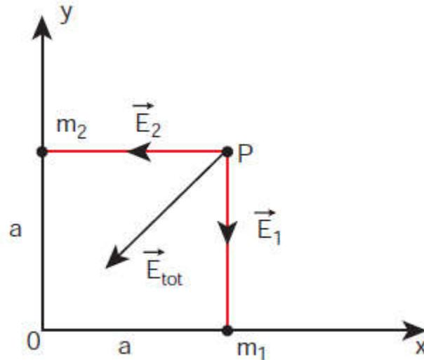
$\vec{E}_{total}$  points towards the origin of the co-ordinate system and the magnitude of  $\vec{E}_{total}$  is  $\frac{Gm}{a^2}$ .
