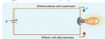
Direction of conventional current and electron flow
