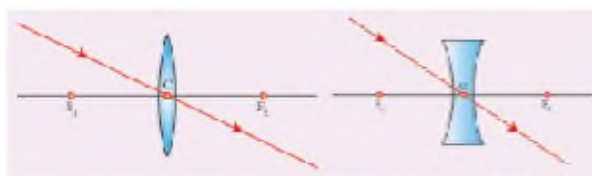
Figure 2.3 Rays passing through the optical centre
