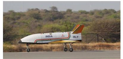
✓ According to ISRO, it was for the first time in the world that a winged body was carried to an altitude of 4.5km by a helicopter and released for carrying out an autonomous landing on a runway.
