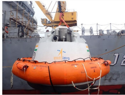
CMRM being lifted onto Ship deck
